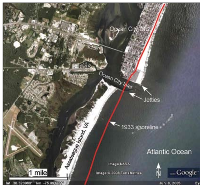
Figure 23. Aerial photograph of Ocean City Inlet, which formed in 1933 (Google Earth; NASA, 2005). The 1933 shoreline is shown in red, the photograph is from 2005. Jetties were built in 1933 and 1934 in an attempt to stabilize the inlet for navigation. The result was a disruption in the sediment transport processes and a large increase in erosion rates (up to 40 feet/year), reduction in island elevation, and loss of critical beach and dune habitats on Assateague Island down-drift of the inlet. The effects extend for approximately 9 miles southward from the inlet.
